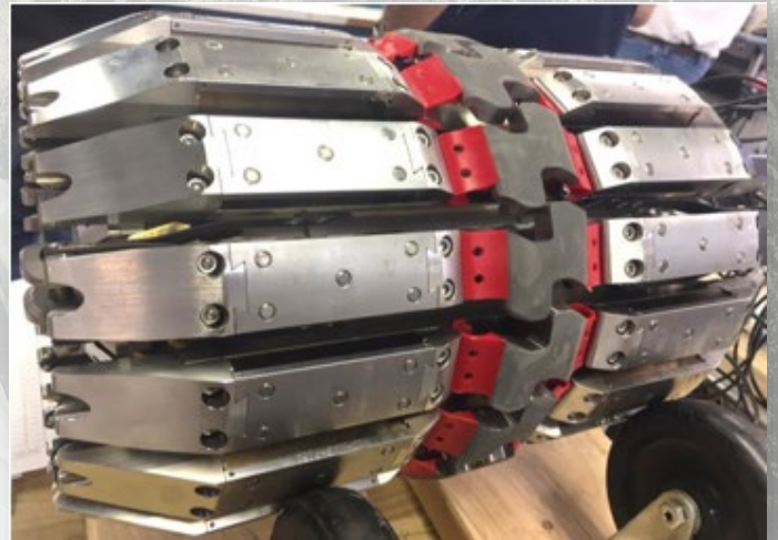
Magnetizer body features 'S shaped' proprietary sensor design
