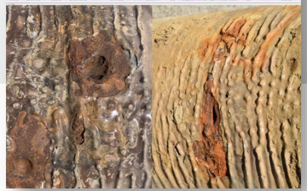
Metal Loss defects at or near girth weld (60% depth)
