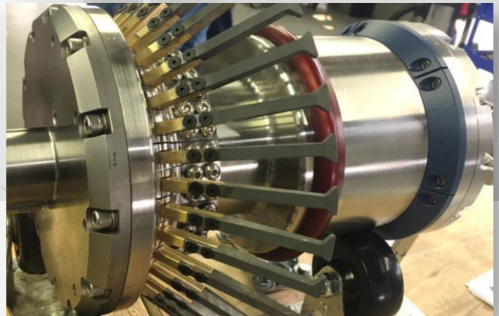
Onboard pipeline geometry assessment (caliper) and onboard Inertial Measurement Unit (IMU) for pipeline XYZ mapping
