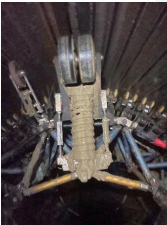
The biofilm, which caused traction problems, was scraped off of the wall and collected on the tool. The collected material is shown on a support spring. The biofilm does not affect the inspection data.
