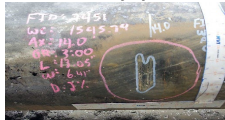
2.05% dent with gouges 15.27% and 24.99%
